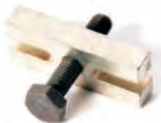
Puller for pretty much any Moped clutch that takes two bolts to remove it
