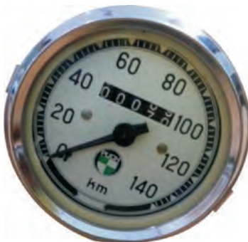
Puch speedometer 80mm PART NO. ZHMS-1717
