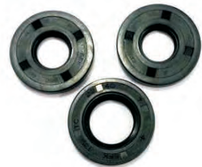
Oil seals for Puch E50 motor. Double lipped seals. One set is comprised of two 17x40x7mm seals and one 22x40x7mm seal.
