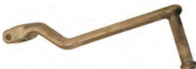
Gear shift Lever (Aluminium casting) Zundapp
