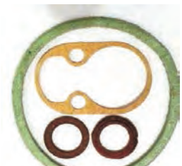
Oil seals for Puch E50 motor. Double lipped seals. One set is comprised of two 17x40x7mm seals and one 22x40x7mm seal.
