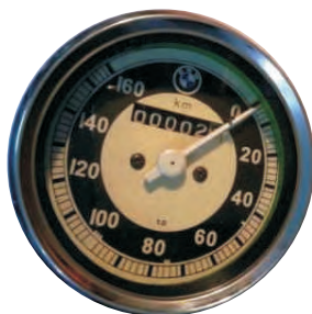
80mm BMW Speedometer R60 R69S R75-5, PART NO. ZHMS-1702
